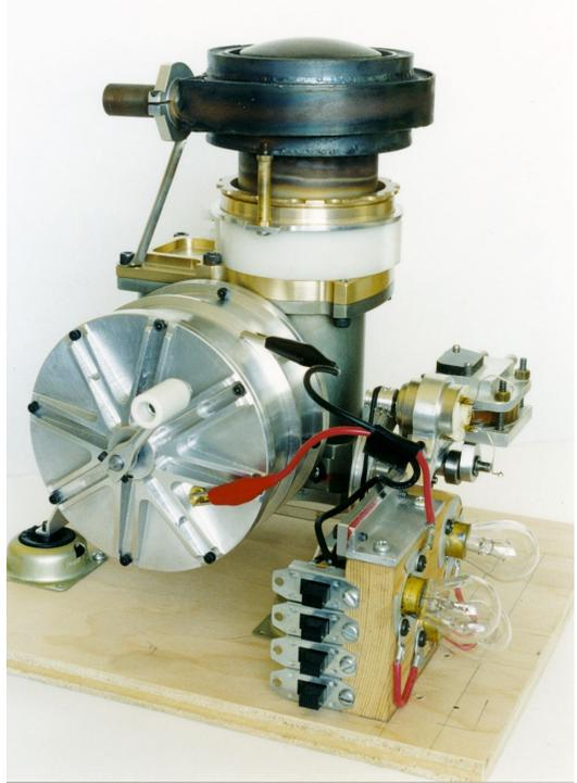
The original D-60 (above left) and the subsequent version with alternator and bulbs (above right). The D-60 cooler, crankshaft, rocking lever, and yoke (below). Opposite: The machine devised to cut the internal fins of the cooler (top), the D-60's piston assembly (bottom left), and the internal fins for the heater (lower right).
