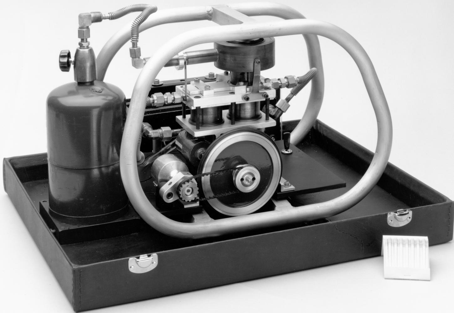
The B-20, as incorporated into a genset by General Pneumatics Corp. (courtesy General Pneumatics Corp.).
