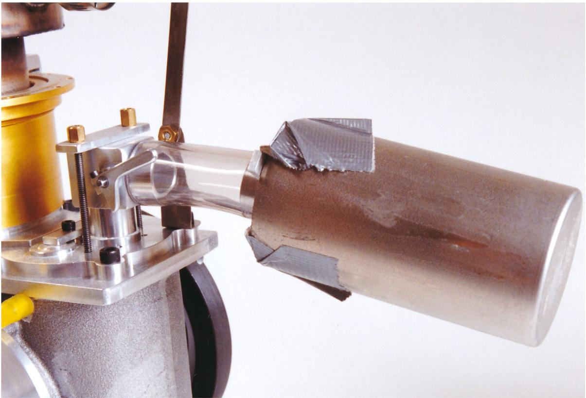
The poppet valved dead volume speed controller (below), and mounted on the D-90 engine (above).
