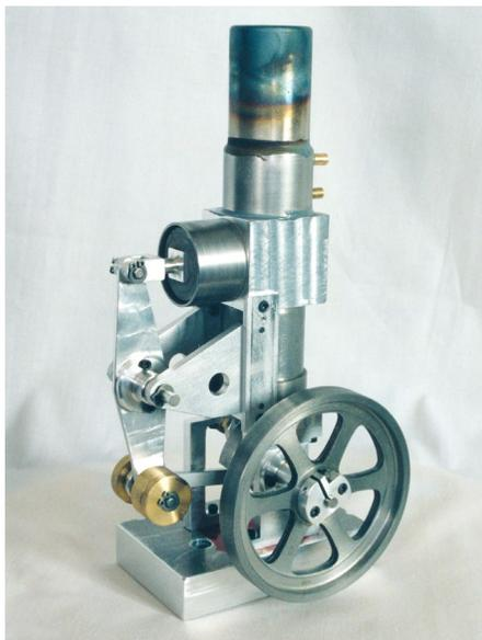
This much-modified engine was the first of the "Rocker-V" type alpha machines. As the name implies, the engine is balanced like a 90° V-twin, and employs a rocking lever to connect the compression piston to the single crankpin.
