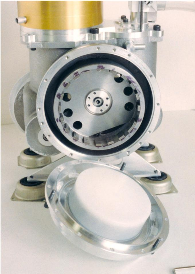
The E-70 engine (above) used the rocking expansion piston and the magnetic shaft drive ideas. Its expansion cylinder did not extend beyond the cooler (upper left), which allowed very close cylinder spacing. The magnetic drive was later adapted to the D-90 engine.
