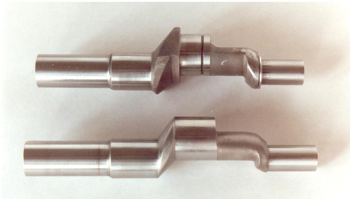
The original shouldered crankshaft is shown above the modified crank that solved the fretting problem (above); the C-60 mounted in a bicycle for testing (below).
