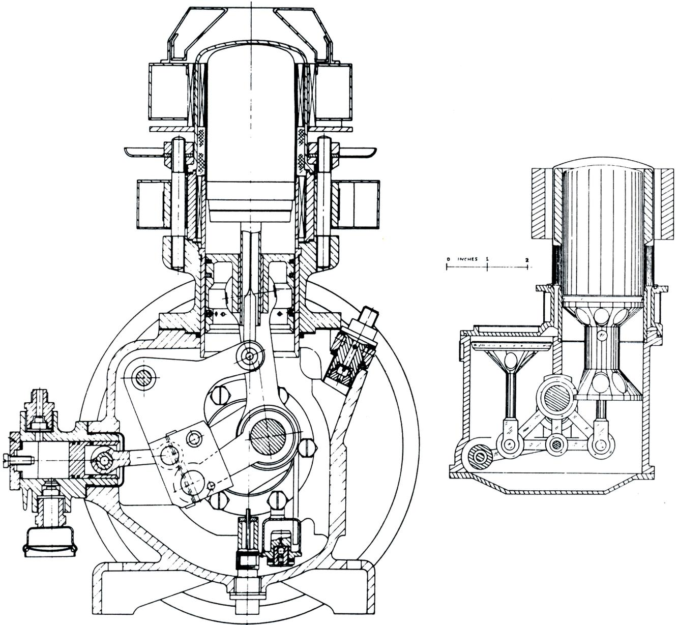
The Philips MP1002CA air engine of about 63cc swept volume (left) is shown on a common scale with the D-60 (right). (drawing of Philips engine courtesy of Professor Allan J. Organ).
