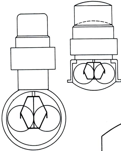
On the left is the 65cc rhombic, with its bore/stroke ratio of 2.125 to 1. On the right is an engine of the same swept volume, but with a bore/stroke ratio of 6 to 1. The dotted line shows the further height reduction possible if the top, rather than the side, of the cylinder cap is made the "heater".
