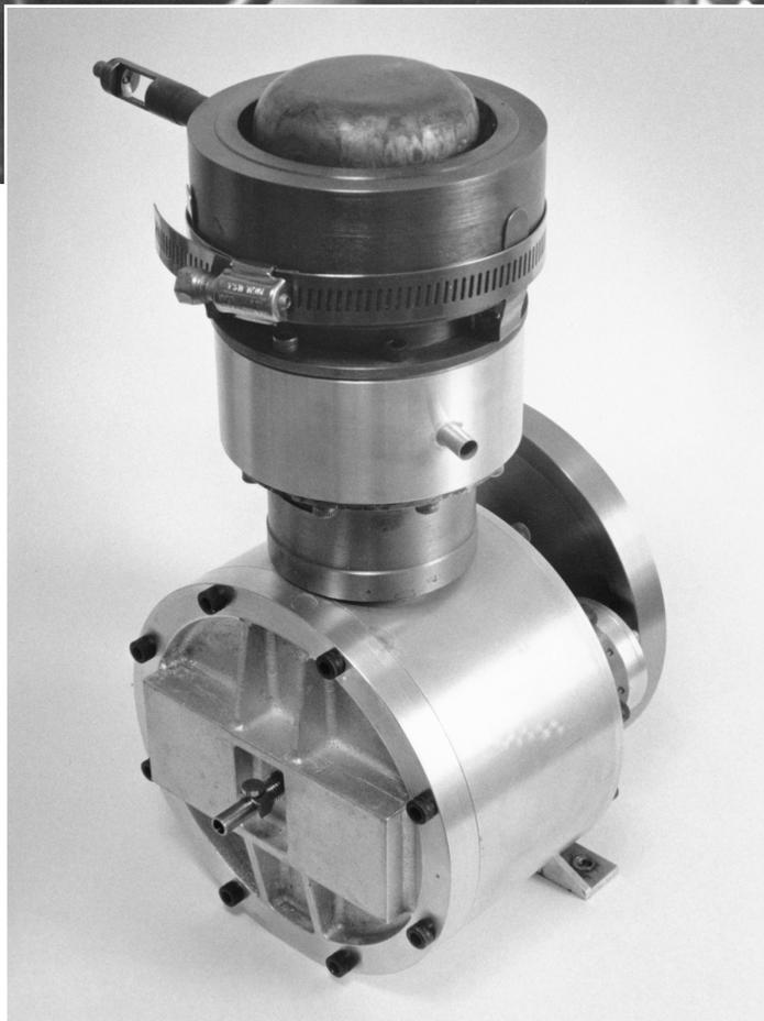
The 65cc rhombic with its first burner on an early brake (above), and in its present form (left).
