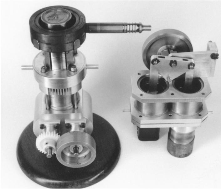
The 15cc alpha with yoke drive, shown with the 11cc rhombic.
